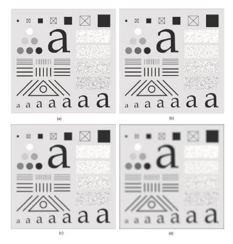
Figure 3: (a) Test pattern of size  $1024 \times 1024$  pixels. (b)-(d) Results of lowpass filtering with box kernels of sizes  $3 \times 3$ ,  $11 \times 11$ , and  $21 \times 21$ , respectively.
