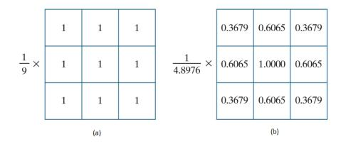
Figure 2: Examples of smoothing kernels: (a) is a box kernel; (b) is a Gaussian kernel.
