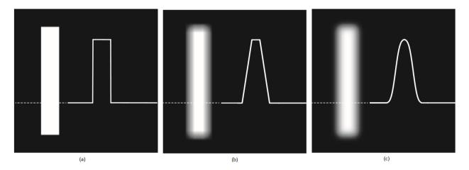
Figure 5: (a) Image of a white rectangle on a black background, and a horizontal intensity profile along the scan line shown dotted. (b) Result of smoothing this image with a box kernel of size  $71 \times 71$ , and corresponding intensity profile. (c) Result of smoothing the image using a Gaussian kernel of size  $151 \times 151$ , with K = 1 and  $\sigma = 25$ . Note the smoothness of the profile in (c) compared to (b).
