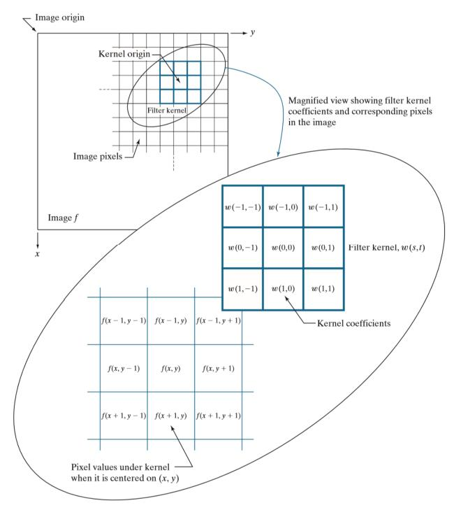
Figure 1: The mechanics of linear spatial filtering using a  $3 \times 3$  kernel. The pixels are shown as squares to simplify the graphics. Note that the origin of the image is at the top left, but the origin of the kernel is at its center. Placing the origin at the center of spatially symmetric kernels simplifies writing expressions for linear filtering.
