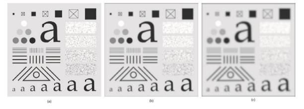
Figure 4: (a)A test pattern of size  $1024 \times 1024$ . (b) Result of lowpass filtering the pattern with a Gaussian kernel of size  $21 \times 21$ , with standard deviations  $\sigma = 3.5$ . (c) Result of using a kernel of size  $43 \times 43$ , with  $\sigma = 7$ . This result is comparable to Fig. 3(d). We used K = 1 in all cases.
